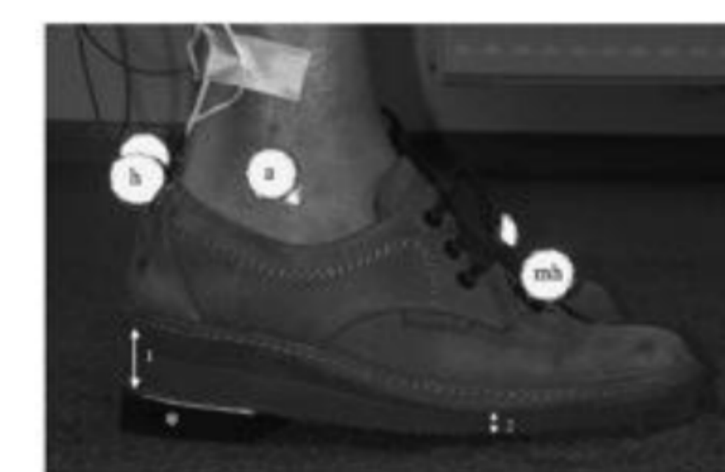
Fig 2. An example of shoes modified by adding a (*) 2-cm high standard heel is shown. The shoe insole is the difference of sole height measured at the (1) heel level and the (2) metatarsal head level. Markers were put on the lateral malleolus (a) over the second metatarsal head (mh) and behind the heel (h).
