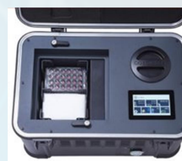
Figure 3. Transportable cell incubator, Cellbox. Graphical representation of the data log exported from the Cellbox® for stationary incubation and transport. The Cellbox was pre-set to 37 °C and 5% CO 2 before the packaged midbrain organoids were transferred to the incubation chamber. The Cellbox® data logging system was activated and the device placed into the packaging kit for overnight incubation. Transport started in the early morning and lasted for approximately 8 hours before the Cellbox® was returned to the pickup location. The data logs were exported to the Cellbox® iOS App and the temperature and CO 2 values represented as a line chart.
