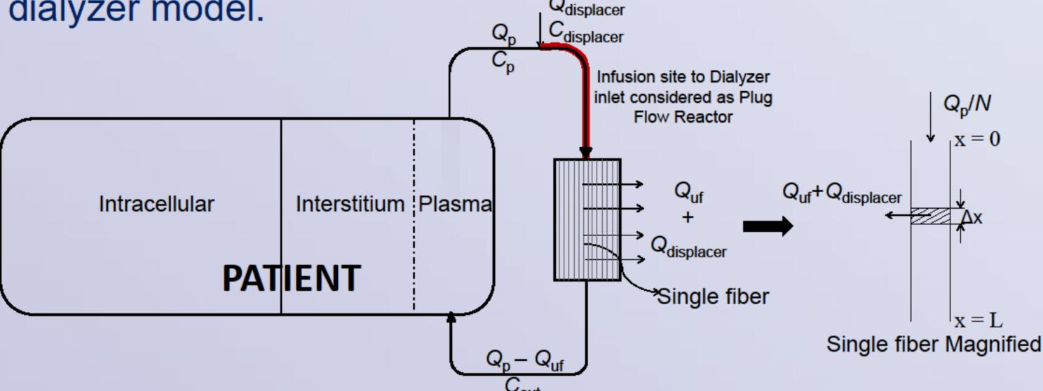
We first tested the model output in a conventional HD setting and confirmed the model reliability based on correct estimation of reduction ratio and total removal.
