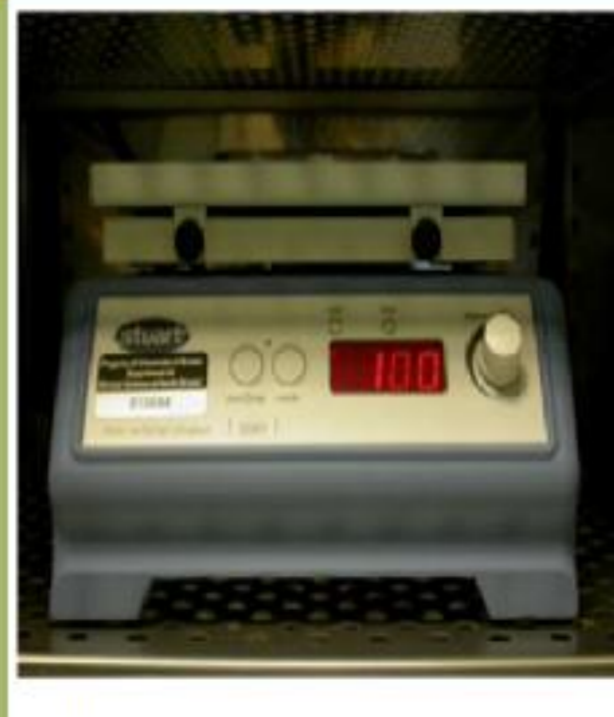
Figure 4: SSM1 Stuart Staffordshire orbital shaker; 75 rpm produce 10dyn/cm 2 of laminar shear stress at the edge of petri-dish used. Equation used \tau_w = \alpha^2 [\rho \eta (2\pi f)^2]
