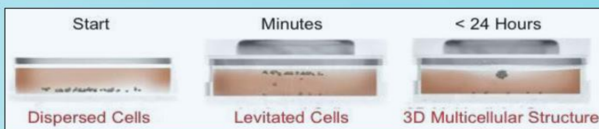
Fig.3: Schematic of the magnetic "bio-assembler". Cells are incubated for 24 hours with "nanoshuttle" which magnetises them. A magnet above the culture flask then allows cells to grow in 3D at the air-liquid interface.
