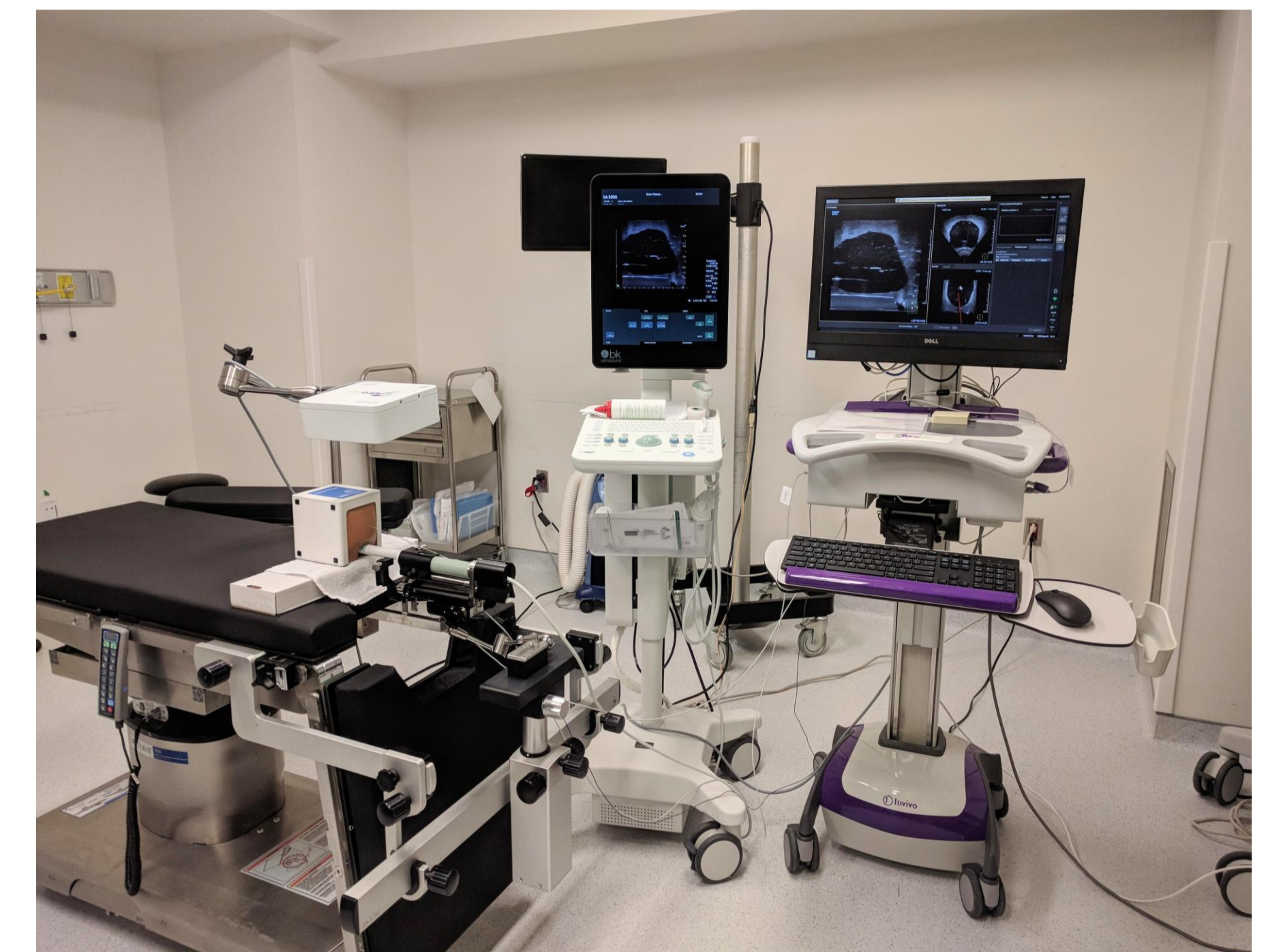
Fig. 1: Setup of the PDMS (Philips Disease Management System) for HDR brachytherapy procedures. Includes the guidance system (right), US scanner (middle) and tracking system.
