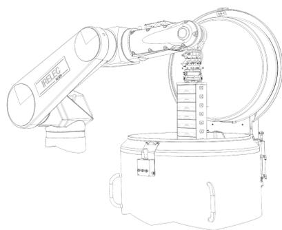
As reliability is the main feature required with automation, IRELEC has built INLANDYS® on reliable **field-proven robotic technologies** and existing commercially-available cryogenic tanks.
