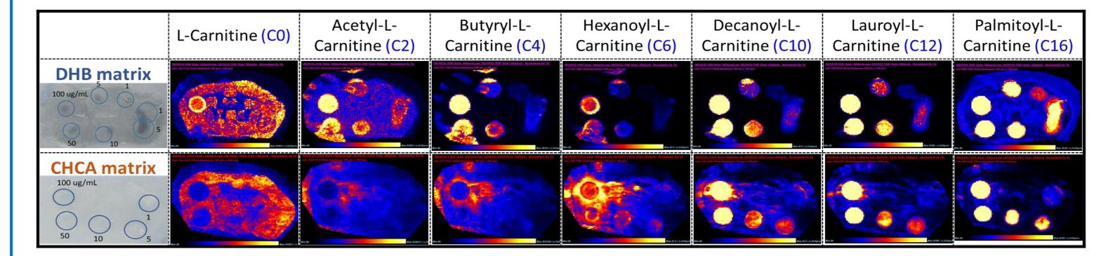
Region of interest (ROI) analysis of standards spots depicted different LoDs depends on FA chain lengths; C16 (< 0.1 μg/mL) > C12 (~0.1 μg/mL) > C10 (~0.2  $\mu g/mL$ ) > C6 (~0.2  $\mu g/mL$ ) > C4 (~1  $\mu g/mL$ ) > C2 (~5  $\mu g/mL$ ) > C0 (~100  $\mu g/mL$ ).
